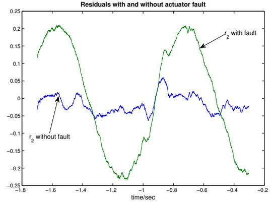
Fig. 3. Residuals  $r_2(t)$  in fault-free case and for an actuator loss of 20%.
