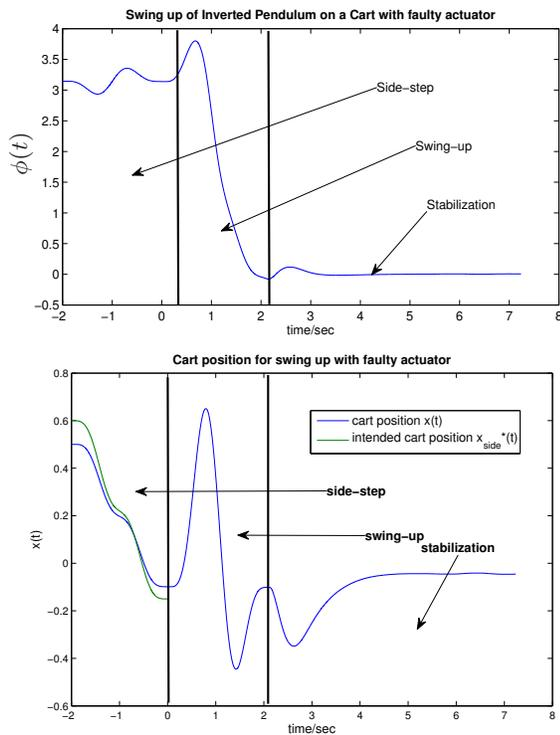
Fig. 5. Side-step, swing-up and stabilization of the pole under faulty conditions: pole angle (top) and cart position (bottom). The actuator loss of 20% was successfully identified during the side-step and could be compensated for later on. The initial cart position is shifted by 0.1m in order to avoid an exceeding of the available rail length.
