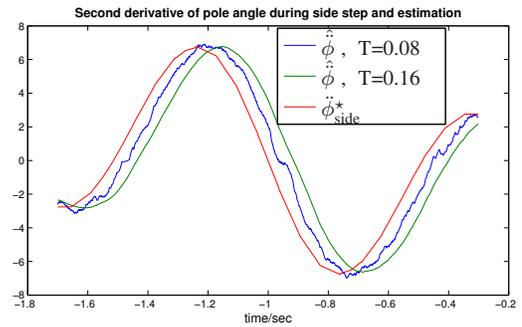
Fig. 4. Second derivative  $\ddot{\phi}_{\text{side}}^*(t)$  and its estimation for  $M = 2$  and two choices for  $T$ . Clearly, increasing  $T$  raises the predicted delay of  $\frac{T}{2}$ , while the noise attenuation improves, see (28) together with (29).
