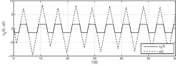
Fig. 4. The time evolutions of the actual control signal  $u_s(t)$  and of  $u(t)$  in the second example
