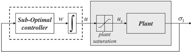
Fig. 1. The scheme of the control system using the original sliding mode controller
