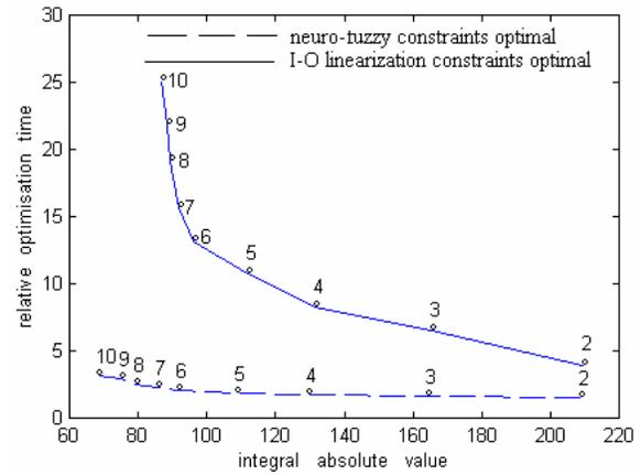
Fig.8 Comparison of controller performance for different prediction horizon.  $H_p = 2, \dots, 10$  for I-O linearization;  $N = 2, \dots, 10$  for neuro-fuzzy.
