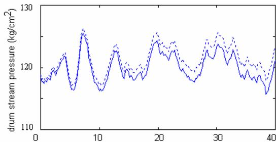
Fig.4 Steam-boiler system(solid line) and IOFL model (dotted line)
