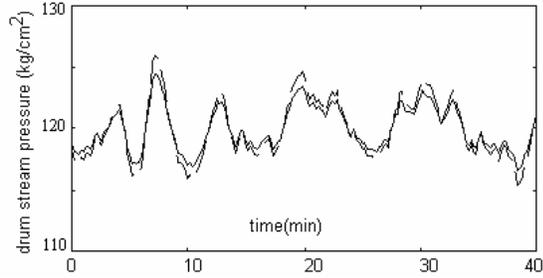
Fig.5 Steam-boiler system(solid line) and neurofuzzy model (dashed line)
