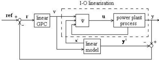
Fig.1. Linear model-based predictive control based on IOFL
