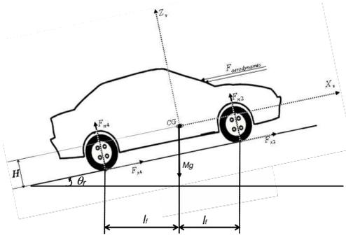
Fig. 2. Vehicle and external forces in slope
