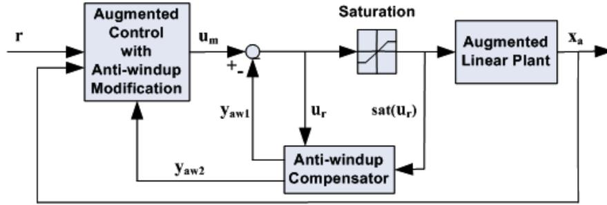
Fig. 4. The nominal control structure with anti-windup compensator for the rate-limited system in the augmented form
