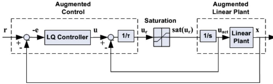
Fig. 3. The rate-limited system including the linear plant and the unconstrained controller
