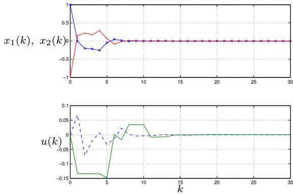
Fig. 2. The behaviors of the states  $x_1(k)$ ,  $\times$ , and  $x_2(k)$ ,  $\cdot$ , (top) and the control signals,  $u_k = Kx_k$ , dashed line, and  $u_{k-d_k} = K_d x_{k-d_k}$ , solid line (bottom).
