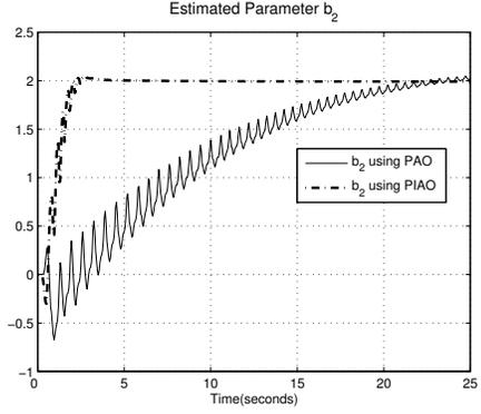
Fig. 7. Estimated  $\hat{b}_2$  using adaptive and PI adaptive observers
