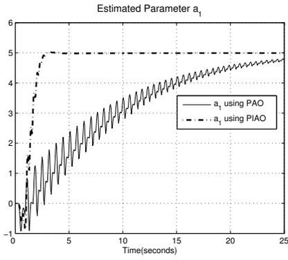
Fig. 4. Estimated  $\hat{a}_1$  using adaptive and PI adaptive observers
