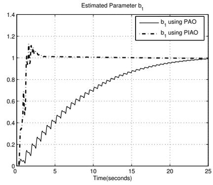
Fig. 6. Estimated  $\hat{b}_1$  using adaptive and PI adaptive observers
