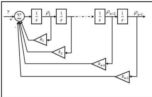
Fig. 1. The Auxiliary Filter Structure
