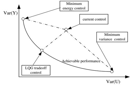
Fig. 2. Performance assessment benchmark with different control objective
