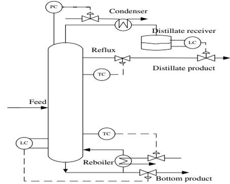
Fig. 4. Schematic diagram of the separation process
