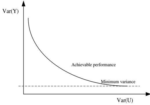
Fig. 1. Optimal performance curve obtained through LQG benchmark
