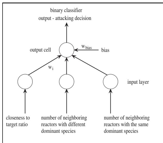
Fig. 3. Binary classifier used in each local controller agent.
