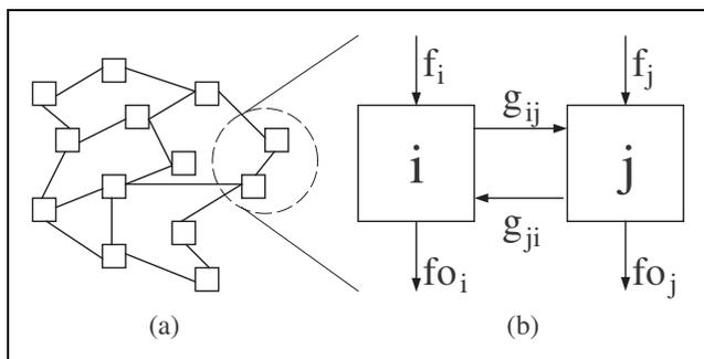
Fig. 1. (a) Network of interconnected reactors. Feed and exit streams are not shown. (b) Detail view of interconnection flows between reactors with feed and exit streams.
