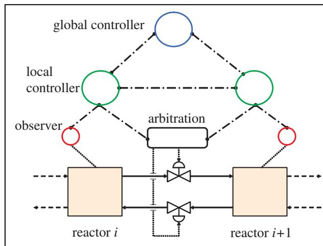
Fig. 2. Hierarchical layers of controller framework.
