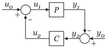
Fig. 4: The standard feedback configuration,  $[P, C]$
