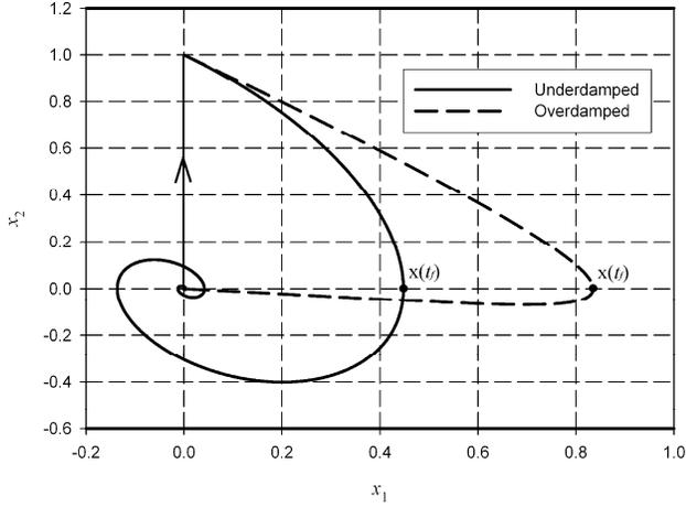
Fig.4. Phase trajectories for instantaneous outflow decrease.
