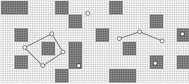
Fig. 1. Example of a movement lattice (light gray squares), nocomm zones (large dark gray squares), and 11  $V_F$  nodes (circles). The lines between nodes indicated edges in  $E_F$ . There are 6 connected components in this figure. Three of the nodes are isolated because they are located inside a nocomm zone.
