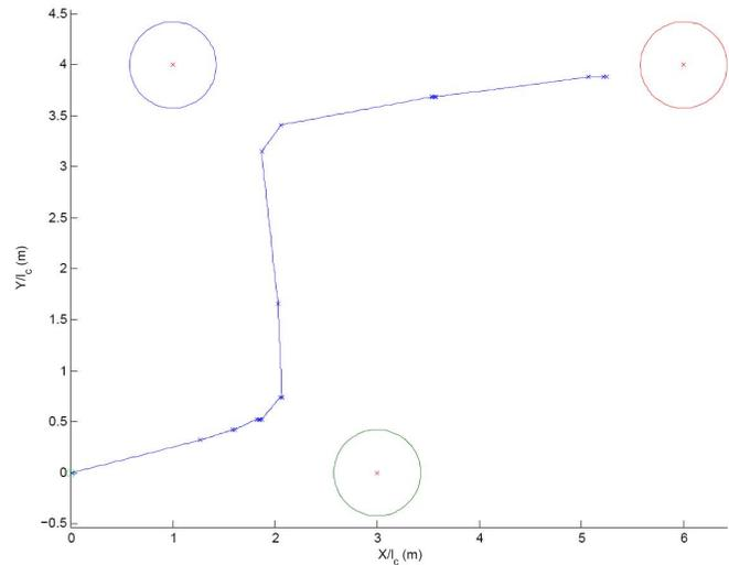
Fig. 1. Optimal flight path for a single UAV
