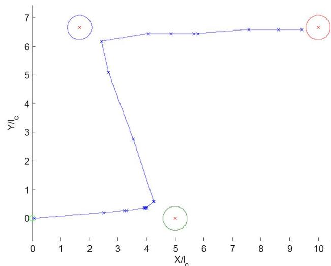
Fig. 2. TSP limiting case - Optimal flight path for a single UAV
