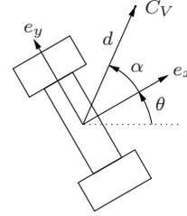
Fig. 1. Vehicle with wheeled mobile dynamics.
