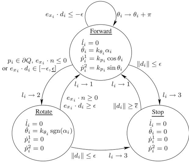
Fig. 2. State transition diagram for each vehicle in the network.
