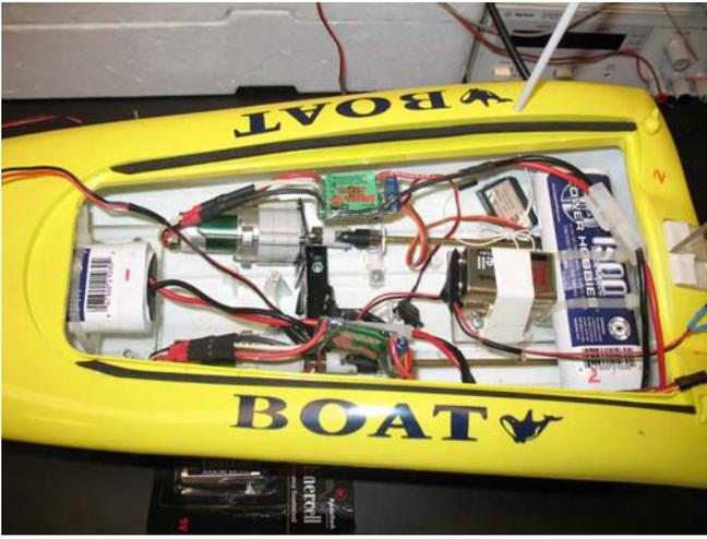
Fig. 2. The vessel with DC motors, receivers, gearboxes, and couplers
