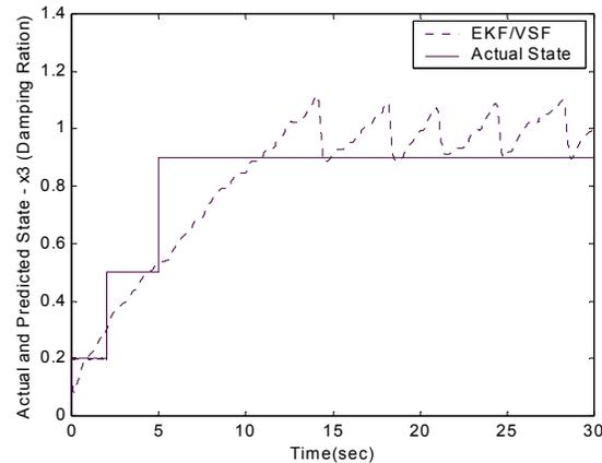
Figure 5b: Estimated and Actual States Associated with Modeling Error and increased boundary layer (x3 - Damping ratio)
