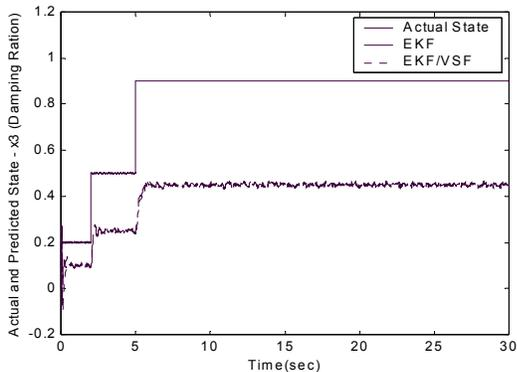
Figure 1c: Estimated and Actual States Associated with State 3 (Damping ratio)
