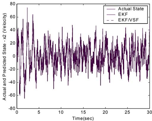
Figure 1b: Estimated and Actual States Associated with State 2 (Velocity)
