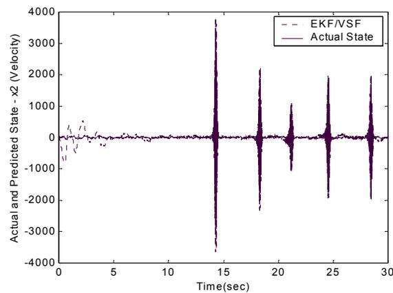
Figure 5b: Estimated and Actual States Associated with Modeling Error and increased boundary layer (x2- Velocity)
