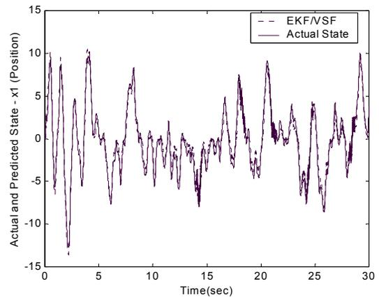
Figure 5a: Estimated and Actual States Associated with Modeling Error and increased boundary layer (x1 - Position)
