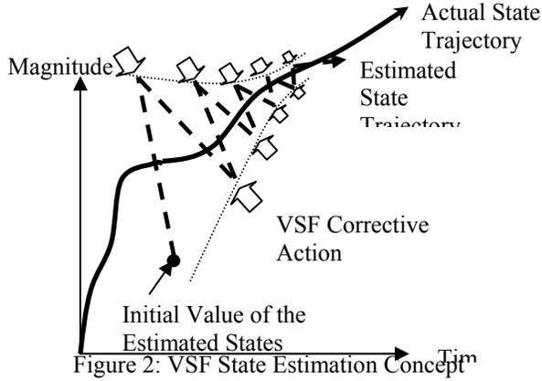
Figure 2: VSF State Estimation Concept
