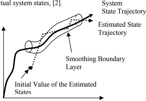
Figure 3: Convergence of the Estimated State Trajectory due to VSF Action
