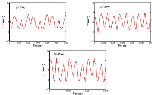
Fig. 11. Time series of error in measured and model displacement of piezoceramic actuator responses at different excitation frequencies.
