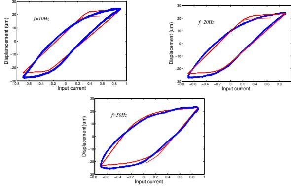
Fig. 6. Comparisons of measured responses of magnetostrictive actuator with the results derived from the generalized rate dependent rate-dependent model under sinusoidal waveform inputs at 10 to 50 Hz different excitation frequencies ( —measured ; - -model).
