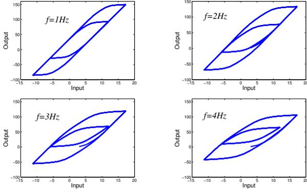
Fig. 4. Simulation results attained from the rate dependent Prandtl-Ishlinskii model of rate dependent play operator at different excitation frequencies.
