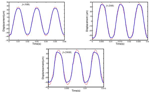
Fig. 10. Time series of measured and model displacement of piezoceramic actuator responses at different excitation frequencies( - - - measured; — model)
