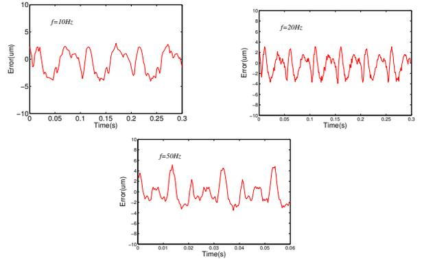
Fig. 8. Time series of error in measured and model displacement of magnetostrictive actuator responses at different excitation frequencies.
