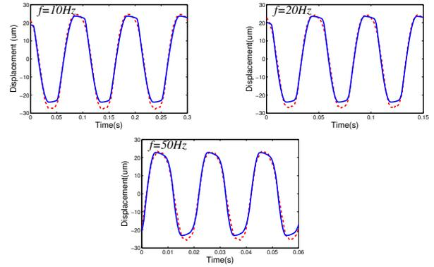
Fig. 7. Time series of measured and predicted displacement of magnetostrictive responses at different excitation frequencies ( —measured ; - -model).
