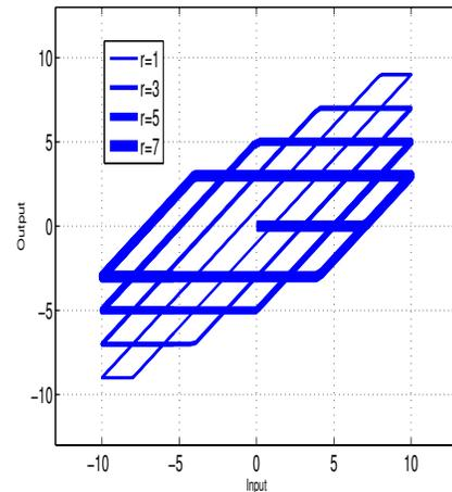
Fig. 2. Influence of threshold  $r$  on the output of the play operator,  $v(t) = 10 \sin(2t)$ .
