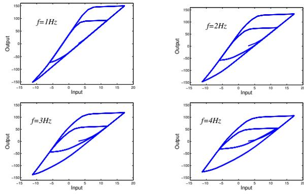
Fig. 5. Simulation results attained from the generalized rate dependent Prandtl-Ishlinskii model of rate dependent play operator at different excitation frequencies.
