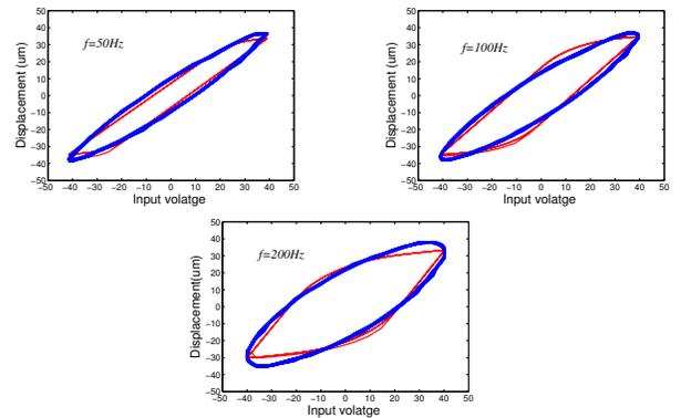
Fig. 9. Comparisons of measured responses of piezoceramic actuator with the results derived from the rate dependent Prandtl-Ishlinskii model under sinusoidal waveform inputs at 10 to 100 Hz different excitation frequencies ( —measured ; - -model).
