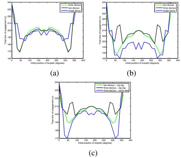
Fig. 11. (a) Multiple same side deployments and single optimum deployment (b) Multiple zig-zag deployments and single optimum deployment (c) Multiple zig-zag deployments and same side deployments
