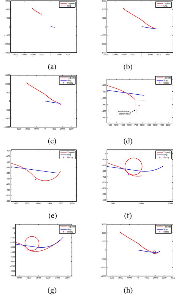
Fig. 4.  $\phi = 135^0$ ,  $t^D = 170.5s$ ,  $\theta = 303^0$ ,  $t_0 = 259$  s (a)  $t=50s$ : Initial stages (b)  $t=169s$ : Before deployment (c)  $t = t^D$  (d)  $t=178s$ : Decoy identification (e)  $t=193s$ : Overshooting of torpedo (f)  $t=234s$ : Reacquiring of ship (g)  $t = t_f$  (h)  $t = t_f$ ; Original scale
