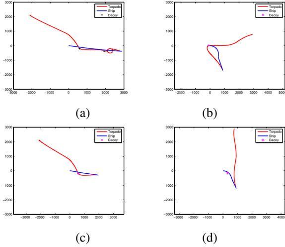
Fig. 5. Some special trajectories (a) Optimum strategy combined with last moment deployment (b)  $\phi = 15^\circ$ ,  $t^D = 0s$ ,  $\theta = 170^\circ$  (c)  $\phi = 135^\circ$ ,  $t^D = 117.68s$ ,  $\theta = 94.5^\circ$  (d)  $\phi = 135^\circ$ ,  $t^D = 170.56s$ ,  $\theta = 303^\circ$
