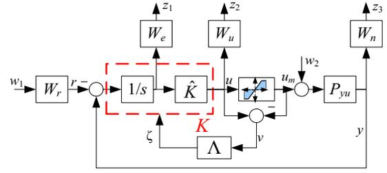
Figure 3: Anti-windup closed loop system
