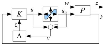
Figure 1: General closed loop system with anti-windup
