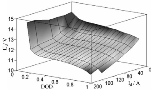
Fig.6. Discharging MAP of NiMH Battery
