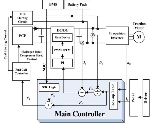
Fig.8. Fuel cell active control system
