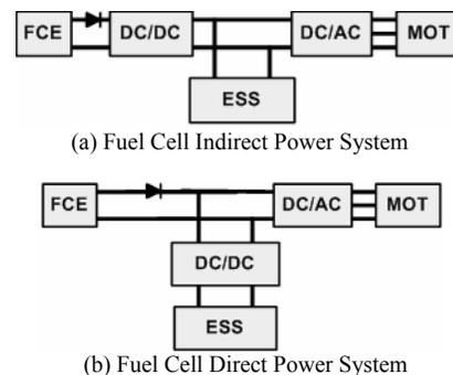
Fig.1 Fuel Cell Hybrid Power System
