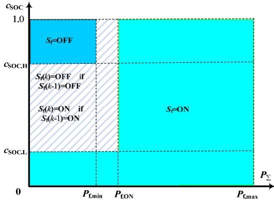
Fig.9. Control Logic for the conventional Fuel cell output power oriented Control Strategy
