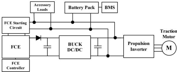
Fig.2. Fuel Cell Hybrid Electric Bus Power Train
