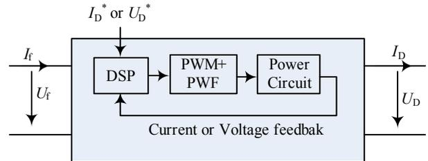
Fig.5. DC/DC converter's control logic
