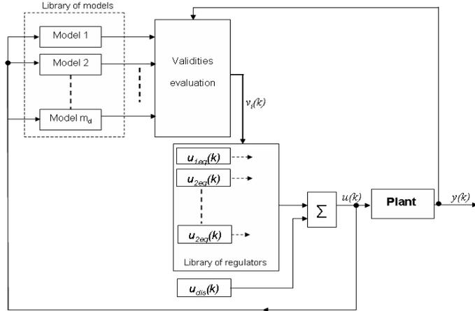
Fig. 8. The structure of a multimodel discrete second order sliding mode control (MM-2-DSMC).
