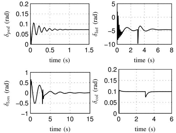
Fig. 4. Control inputs of the Eagle RUAV computed at sampling time 0.02 seconds
