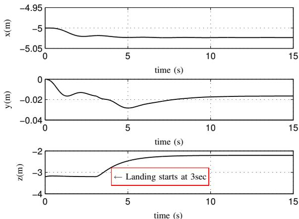
Fig. 3. Cartesian state  $\zeta = [x, y, z]^T$  of the Eagle RUAV computed at sampling time 0.02 seconds. The landing operation starts after 3 seconds of the simulation time.
