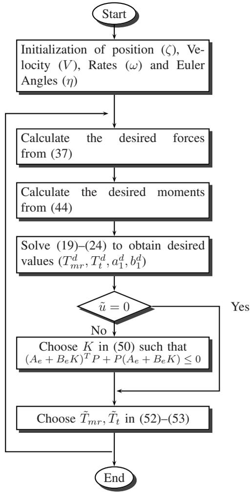
Fig. 2. Backstepping-based controller flow chart for the Eagle RUAV. The flow chart explains a step-wise procedure to obtain the RUAV control inputs. The controller uses a novel result to provide a correction for the flapping dynamics due to higher DOF system.
