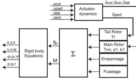
Fig. 1. Block diagram of a Rotary wing UAV dynamics
