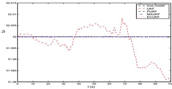
Fig. 4. Total density  $\Sigma\rho$  obtained using the estimates from UKF, ECUKF, PUKF, and MAUKF. ECUKF, PUKF, and MAUKF provide estimates that ensure that the estimates satisfy the constraint. However, since no constraints are enforced in UKF, the total density or the total energy is not conserved.
