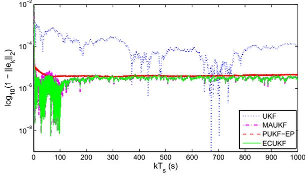
Fig. 1. Estimation errors of the quaternion vector norm using UKF, ECUKF, PUKF-EP, and MAUKF algorithms. ECUKF and MAUKF estimates almost coincide.
