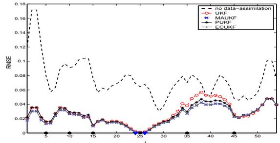
Fig. 3. RMS energy-estimate error at each cell  $i$ . The error when no data assimilation is performed is also shown for comparison. The performance of ECUKF, PUKF, and MAUKF is better than the performance of UKF. The performance of MAKF and ECUKF is very similar because the constraints are linear with respect to the state. The cells where disturbance enters the system is indicated by ' $\bullet$ ' and the cells where measurements are available is indicated by ' $\blacktriangledown$ '.
