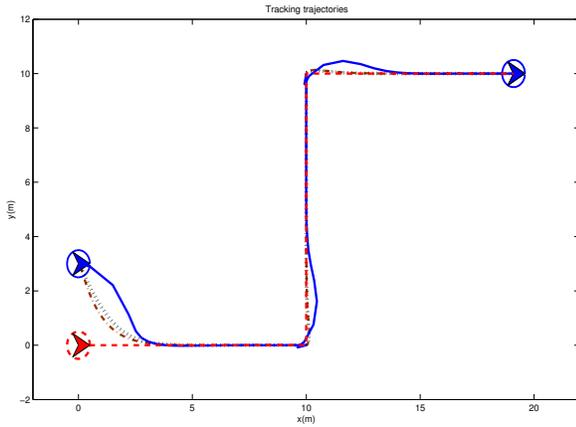
Fig. 3. Tracking trajectories. Dashed: Reference. Solid: FSC-MPC. Dotted: Samson. Dash-dot: Kanayama.
