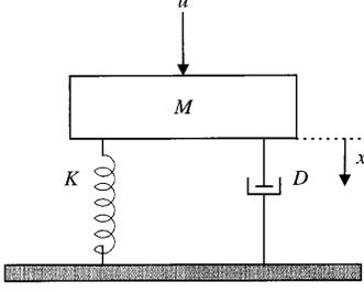
Fig. 1. Nonlinear mass-spring-damper system.
