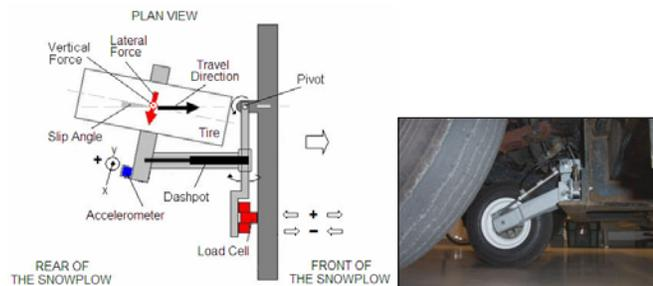
Fig. 2. Wheel Based System
