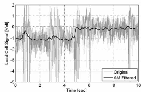
Fig. 3. Typical Force Signal
