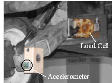
Fig. 7. Accelerometer and Load Cell Locations
