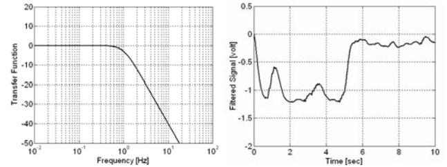
Fig. 5. 2nd Order Butterworth Low Pass Filter and the Filtered Signal
