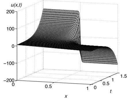
Fig. 1. Finite time blow-up of open-loop system (with constant inputs (4)) for  $\sigma = 3$  and  $u_0(x) = U(0) + 2 + (U(1) - U(0) - 4)x$ .
