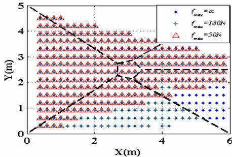
Fig 3. Workspace when the end-effector's orientation is zero ( $\Delta$  points:  $f_{max}=50N$ , + points:  $f_{max}=180N$ ,  $\bullet$  points: without tension limit), by linear algebra, cable robot 1.
