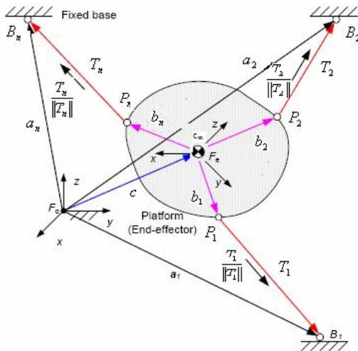
Fig.1. General kinematics of a cable robot
