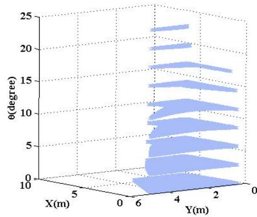
Fig 4. Workspace when the end-effector's orientation is variable, cable robot 1.
