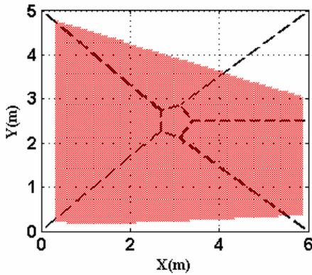
Fig 2. Workspace when the end-effector's orientation is zero, by variant of Bland's pivot rule, cable robot 1.
