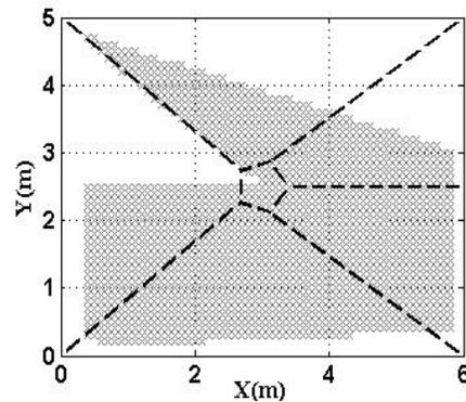
Fig 5. Workspace when the end-effector's orientation is zero, by direct analysis method, cable robot 1.
