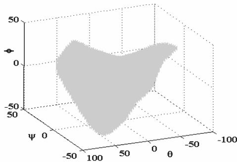
Fig 9. Workspace when the end-effector's position is fixed, cable robot 2. where  $\psi$  rotation about  $x$ ,  $\theta$  rotation about  $y$ ,  $\phi$  rotation about  $z$ .
