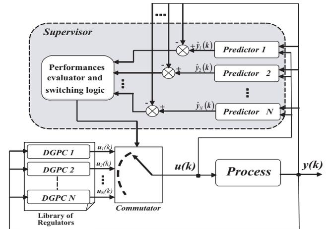
Fig. 4. A general architecture for multimodel switching control with supervisor.
