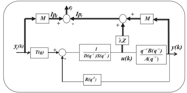
Fig. 1. The Direct Adaptive Generalized Predictive Control structure.
