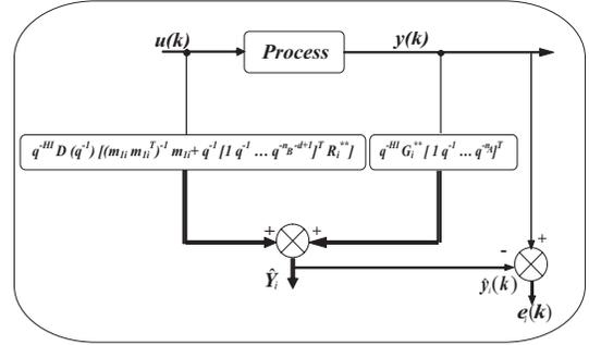
Fig. 5. The proposed local predictor structure.
