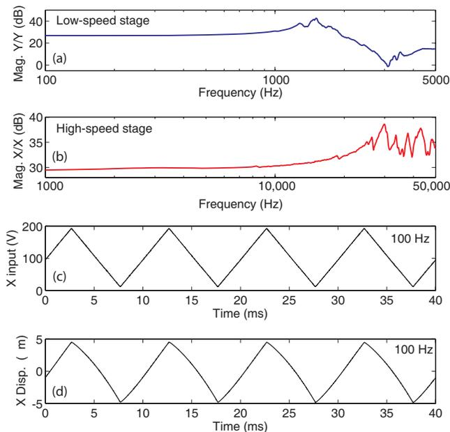
Fig. 7. The measured frequency response of the (a) low- and (b) high-speed stage (units in nm/V). The open-loop (c) input voltage and (d) measured displacement versus time for scanning in the  $x$  direction at 100 Hz.
