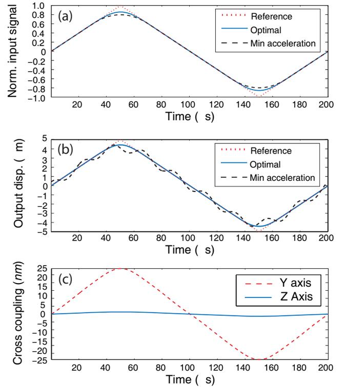
Fig. 5. (a) The scanner input signals: triangular, optimal, and minimum acceleration. (b) The simulated scanner displacement for the optimal and minimum acceleration input. (c) The  $y$ - and  $z$ -axis runout due to the  $x$ -axis trajectory shown in (b).
