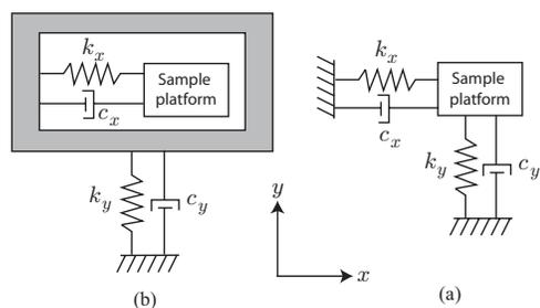
Fig. 1. Configurations for two-axis scanning: (a) serial and (b) parallel kinematics arrangement. The spring constants  $k_x$  and  $k_y$  include the stiffness of the piezoactuators and added flexures in each direction.
