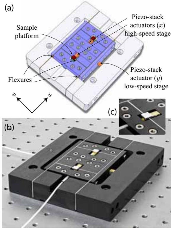
Fig. 3. (a) An assembly drawing of the two-axis high-speed scanner, where the high-speed stage ( $x$ ) is nested inside of the low-speed stage ( $y$ ). (b) A photograph of a manufactured scanner with black surface finish. (c) A close-up view of sample platform and  $x$ -axis piezo-stack actuator.
