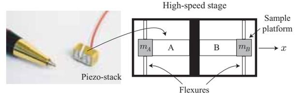
Fig. 2. (Left) A photograph of the piezo-stack actuator and (Right) a sketch of the flexure-guided high-speed stage, where an opposing piezo-stack is used to compensate for the sample platform's inertial effects. These effects can induce unwanted movement on the low-speed ( $y$ -axis) stage.
