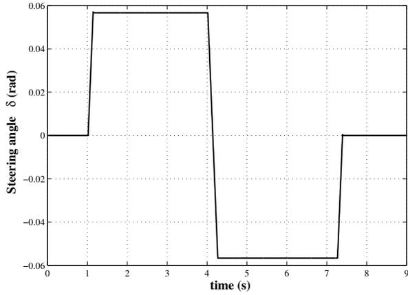
Fig. 4. Steering angle reversal test input corresponding to 50° handwheel angle
