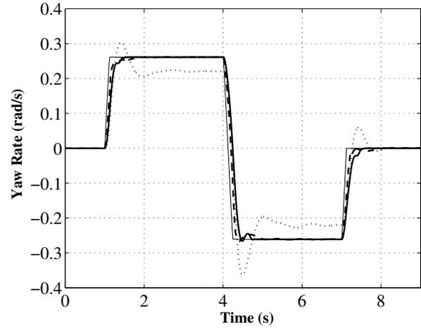
Fig. 6. 50° steer reversal test at 100 km/h, nominal conditions. Comparison between the reference yaw rate course (thin solid line) and the ones obtained with the uncontrolled (dotted) vehicle and the IMC (dashed) and Sliding Mode (solid) controlled vehicles.
