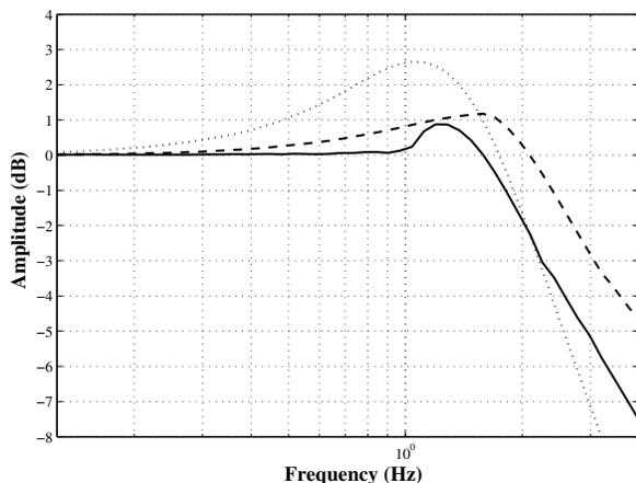
Fig. 9. Steering wheel frequency sweep at 100 km/h. Frequency response: uncontrolled vehicle (dotted), controlled vehicle with IMC (dashed) and Sliding Mode (solid)
