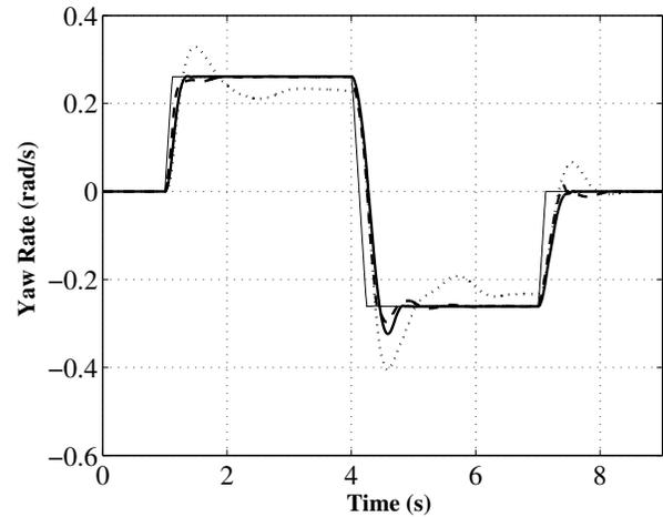
Fig. 7. 50° steer reversal test at 100 km/h with increased vehicle mass. Comparison between the reference yaw rate course (thin solid line) and the ones obtained with the uncontrolled (dotted) vehicle and the IMC (dashed) and Sliding Mode (solid) controlled vehicles.
