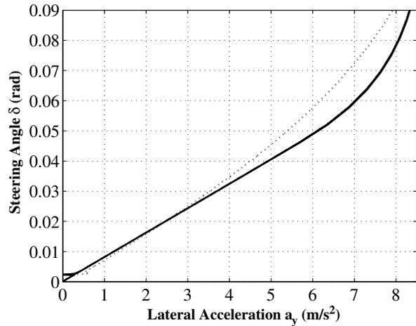
Fig. 5. Steering pad test at 90 km/h: comparison between the reference (thin solid line) steering diagram and the ones obtained with the uncontrolled vehicle (dotted) and with IMC (dashed) and the Sliding Mode (solid) controlled vehicles.
