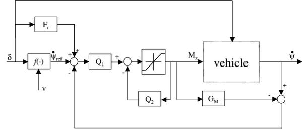
Fig. 3. The proposed control scheme for IMC control system.
