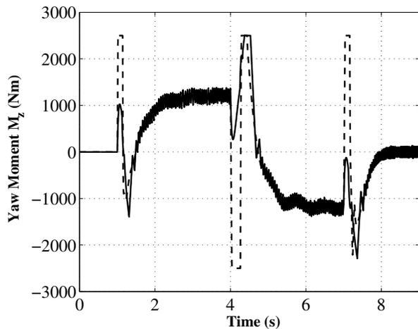
Fig. 8. 50° steer reversal test at 100 km/h, nominal conditions. Comparison between the yaw moment courses obtained with the IMC (dashed) and Sliding Mode (solid) controllers.
