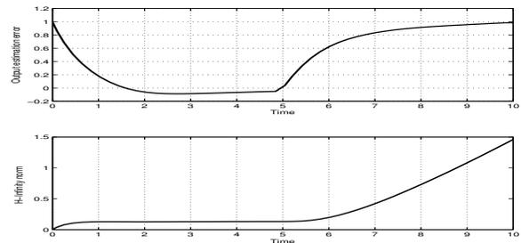
Fig. 2. **Above.** Graph of the output  $H_\infty$  estimation error  $z(t) - z_f(t)$  corresponding to the estimate  $x_f(t)$  satisfying the equations (27)–(28), in the simulation interval  $[0,10]$ . **Below.** Graph of the noise-output  $H_\infty$  norm corresponding to the shown output  $H_\infty$  estimation error, in the simulation interval  $[0,10]$ .
