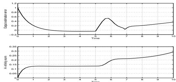
Fig. 3. **Above.** Graph of the output  $H_\infty$  estimation error  $z(t) - z_f(t)$  corresponding to the estimate  $x_f(t)$  satisfying the equations (24),(29), in the simulation interval  $[0,10]$ . **Below.** Graph of the noise-output  $H_\infty$  estimation error, in the simulation interval  $[0,10]$ .
