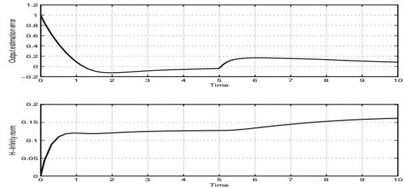
Fig. 1. **Above.** Graph of the output  $H_\infty$  estimation error  $z(t) - z_f(t)$  corresponding to the estimate  $x_f(t)$  satisfying the equations (24)–(26), in the simulation interval  $[0,10]$ . **Below.** Graph of the noise-output  $H_\infty$  norm corresponding to the shown output  $H_\infty$  estimation error, in the simulation interval  $[0,10]$ .
