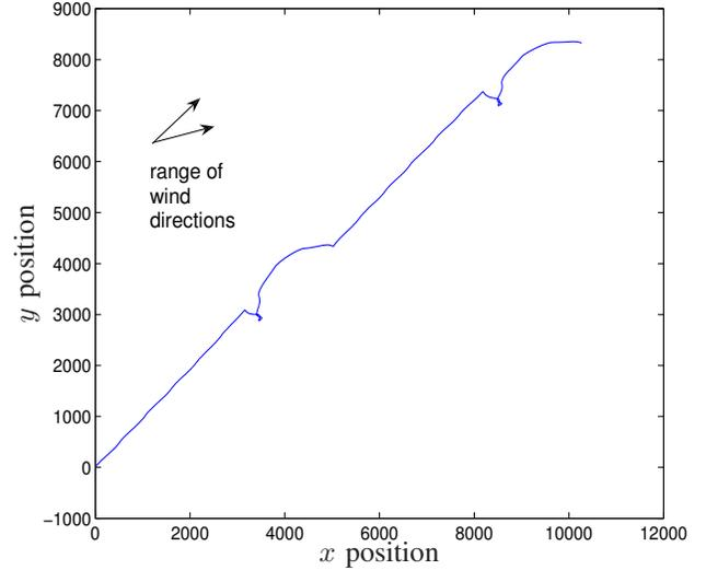
Fig. 3. Flight path of the aircraft in the presence of wind disturbance. The steering angle is an alternating sequence of zeros and ones, which represents the aircraft flying in a straight lines and in circles alternately. The two arrows show the extremities of the wind direction, which is a time-varying triangular waveform.
