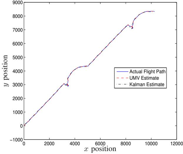
Fig. 4. Actual flight path and estimate of the flight path using the Kalman filter and the unbiased minimum-variance filter in the presence of an unknown wind disturbance.
