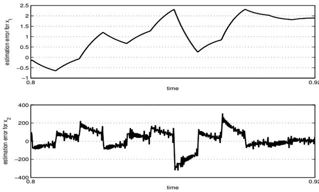
Fig. 2. Graph of the error between the real state  $x_1(t)$  satisfying the first equation in (24) and the optimal filter estimate  $m_1(t)$  satisfying the first equation in (26), graph of the error between the real state  $x_2(t)$  satisfying the second equation in (24) and the optimal filter estimate  $m_2(t)$  satisfying the second equation in (26), on the simulation interval  $[0.80, 0.92]$ .
