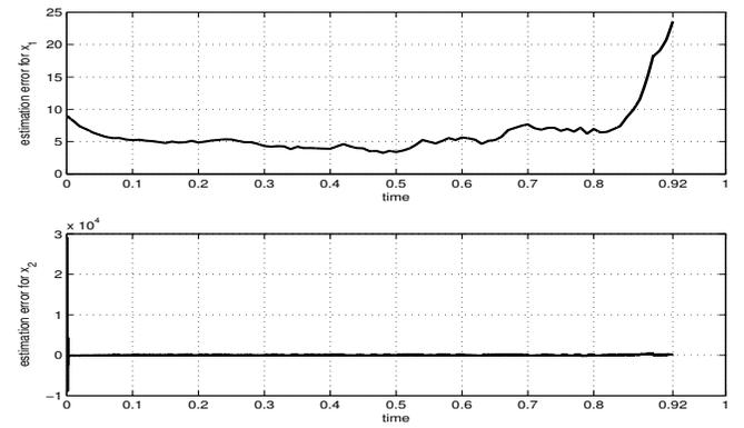
Fig. 5. Graph of the error between the real state  $x_1(t)$  satisfying the first equation in (24) and the estimate  $m_{K1}(t)$  satisfying the first equation in (30), and graph of the error between the real state  $x_2(t)$  satisfying the second equation in (24) and the estimate  $m_{K2}(t)$  satisfying the second equation in (30), on the entire simulation interval  $[0, 0.92]$ .
