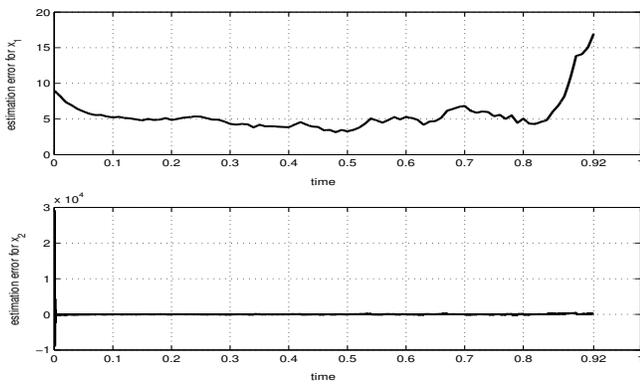
Fig. 3. Graph of the error between the real state  $x_1(t)$  satisfying the first equation in (24) and the estimate  $m_{I1}(t)$  satisfying the first equation in (28), and graph of the error between the real state  $x_2(t)$  satisfying the second equation in (24) and the estimate  $m_{I2}(t)$  satisfying the second equation in (28), on the entire simulation interval  $[0, 0.92]$ .
