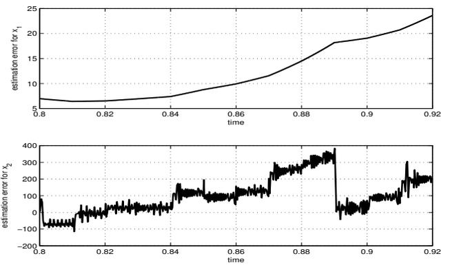
Fig. 6. Graph of the error between the real state  $x_1(t)$  satisfying the first equation in (24) and the estimate  $m_{K1}(t)$  satisfying the first equation in (30), and graph of the error between the real state  $x_2(t)$  satisfying the second equation in (24) and the estimate  $m_{K2}(t)$  satisfying the second equation in (30), on the simulation interval  $[0.80, 0.92]$ .
