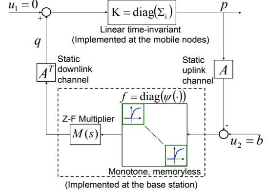
Fig. 2. Block-diagram decomposition of the passivity-based power allocation mechanism presented in [1] and [2]. Exogenous inputs  $u_1$  and  $u_2$  are set to 0 and  $b$  respectively, where the choice of  $b$  is as per the base station administrator. The feedback nonlinearity  $f(\cdot)$  is repeated monotone single-input single-output (SISO). [2] synthesizes a dynamic feedback nonlinearity at the base station by multiplying the output of  $f(\cdot)$  by a Zames-Falb multiplier  $M(s)$ .
