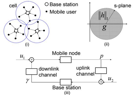
Fig. 1. (i): Cellular network has one base station per cell; a mobile node transmits data to only one base station. (ii) The Nyquist plot of a Zames-Falb multiplier  $m(\cdot) = \delta(\cdot) + h(\cdot)$ . [2] uses the Zames-Falb multipliers to improve the performance of the system shown in (iii).
