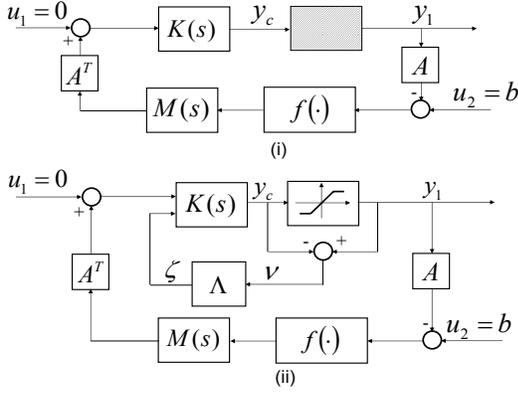
Fig. 3. (i): A prerequisite for the stability results established in [1] is that controller output  $y_c$  does not exceed  $p_{max}$ , which is left uncharacterized. In practice, an upper bound  $p_{max}$  is invariably imposed on  $y_c$ . The shaded block represents a saturation nonlinearity that captures this constraint. (ii) A block diagram representation of the single cell after incorporating our proposed two degrees-of-freedom anti-windup controller.
