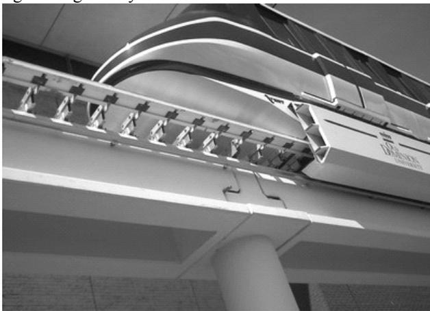
Figure 1 ODU Maglev Vehicle on Guideway
