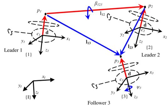
Fig. 3. Formation Parameters of Three Neighboring Helicopters
