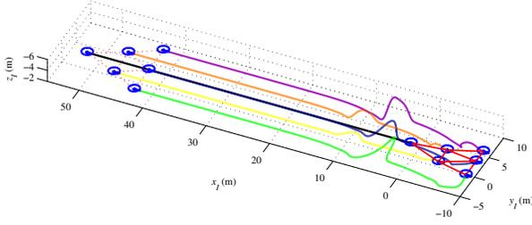
Fig. 4. Triangular Formation Maneuver of 6 Helicopters
