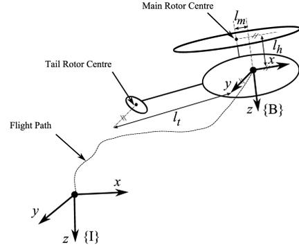
Fig. 1. The Spatial Configuration of the Helicopter
