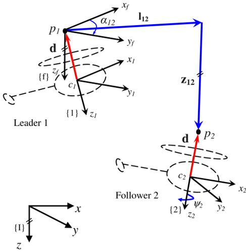
Fig. 2. Formation Parameters of Two Neighboring Helicopters
