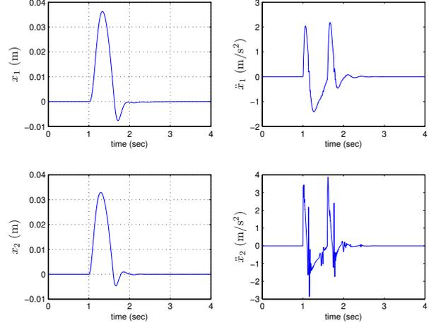
Fig. 4. Responses of sprung and unsprung masses under bump excitation
