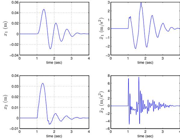
Fig. 6. Responses of sprung and unsprung masses under bump excitation for  $\nu = 0$
