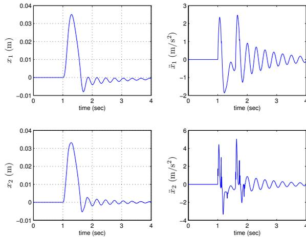
Fig. 7. Responses of sprung and unsprung masses under bump excitation for  $\nu = 2$
