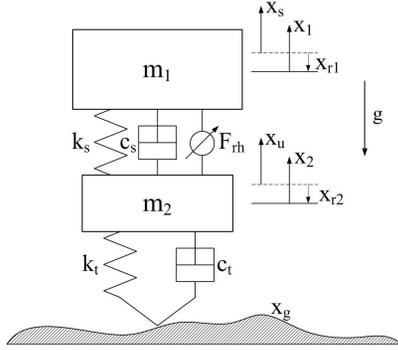
Fig. 1. Quarter Vehicle Suspension model
