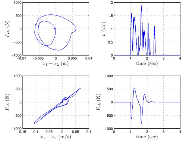
Fig. 5. Damping force and input voltage of MR damper
