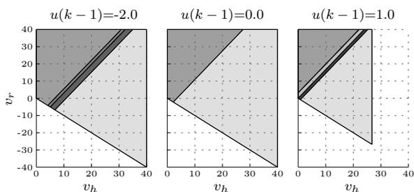
Fig. 4. Three 2D crosscuts of the solution space at constant  $x_r = 10$  m with varying  $x_{e,4} = u(k-1) \in \{-2.0, 0.0, 1.0\}$  m s<sup>-2</sup>.
