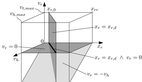
Fig. 3. Visualization of a 3D crosscut of the state-space  $x_e(t)$  at constant  $x_{e,4} = u(k-1)$ . The state-space is bounded by  $\mathcal{B}$ .
