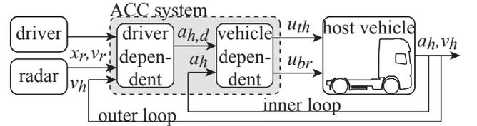
Fig. 2. Schematic representation of the ACC S&G control loop. The ACC S&G system is divided into a generic, outer control loop determining the desired acceleration  $a_{h,d}$  and a vehicle specific, inner control loop determining the actual throttle and brake control signals  $u_{th}$ ,  $u_{br}$  respectively.
