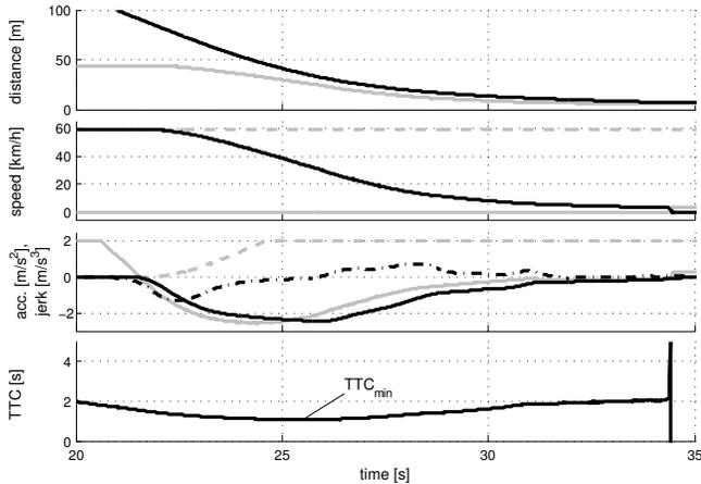
Fig. 6. Experimental results of the approach of a standstill vehicle. The solid black plots represent  $x_r$ ,  $v_h$ ,  $a_h$  and  $TTC$ . The solid grey plots represent  $x_{r,d}$ ,  $v_t$  and the corresponding  $a_{h,d} = a_{h,ACC,d}$ . The dashed grey plots represent  $v_{CC}$  and the corresponding  $a_{h,d} = a_{h,CC,d}$ . The jerk is shown in dash-dotted black on the same scale as the acceleration.
