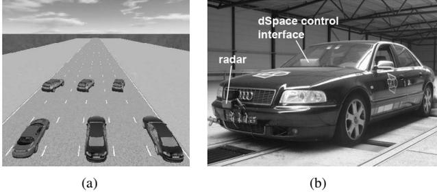
Fig. 5. (a): Screenshot of a PreScan simulation environment. Three ACC S&G-equipped host vehicles and three target vehicles causing corresponding cut-in situations are shown. The ACC S&G systems of the host vehicles are tuned distinctively for comparison. (b): The Audi S8 in which the ACC S&G is implemented. The functionality of the controller was first tested in the TNO VEHIL test facility [24] before the tests in actual traffic have been performed.
