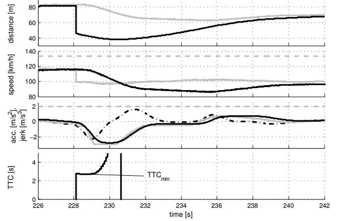
Fig. 7. Experimental results of a cut-in situation (at about 228 s). See Fig. 6 for explanation of the plots.
