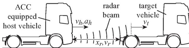
Fig. 1. Example of the ACC working principle; the host vehicle is equipped with an ACC system, which assures automatic following of the preceding target vehicle at a distance  $x_r = x_{r,d}$ . The corresponding radar measures the relative distance  $x_r$  and relative velocity  $v_r$  between the two vehicles.
