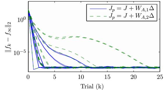
Fig. 5: Convergence of the command signal with  $R, S \rightarrow 0$ .
