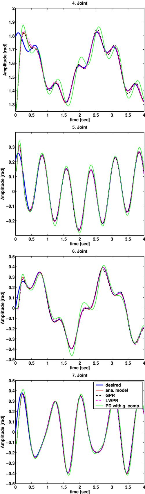
Fig. 5: Tracking performance for joint 4, 5, 6 and 7 with feedforward control using test trajectory.
