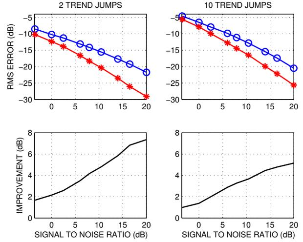
Fig. 2. The upper plot shows RMS error in dB for the monotonic filter (curves marked by \*) and EWMA (curves marked by o). The lower plots show improvement in dB.
