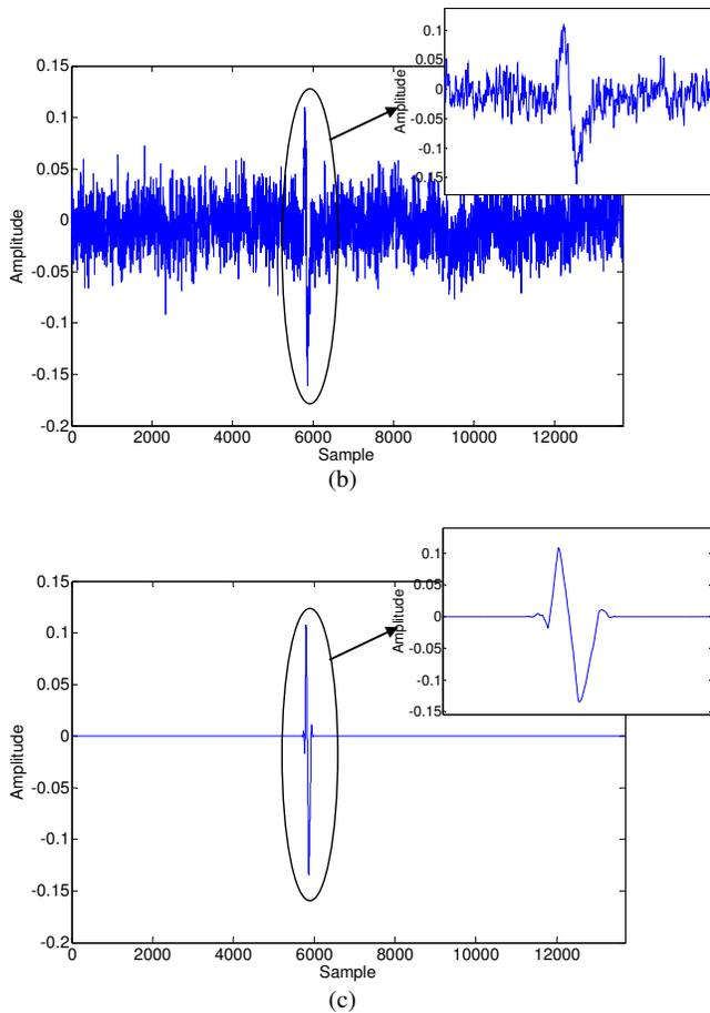
Figure.10 a) Measured signal mixture, b) Interference removal result obtained using ALE, and c) Result obtained after threshold de-noising the ALE output shown in part (b) (Particle: ferromagnetic, diameter =125  $\mu\text{m}$ , shaker frequency = 500 Hz)
