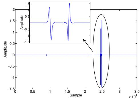
Fig. 8 Threshold de-noised version of the ALE result shown in fig. 7b (Particles: ferromagnetic, diameter = 175  $\mu\text{m}$  and non-ferromagnetic, diameter = 508  $\mu\text{m}$ )
