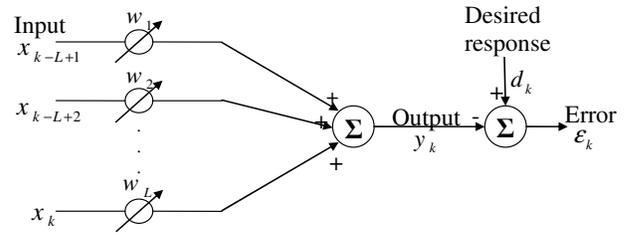
Fig. 5. Adaptive linear filter
