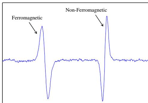
Fig. 2. Sensor output in response to the passage of a metallic particle
