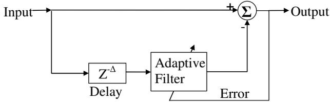
Fig. 6. Adaptive Line Enhancement technique
