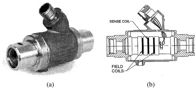
Fig. 1. (a) Oil debris sensor (b) Sensor cross section (Miller and Kitaljevich 2000)
