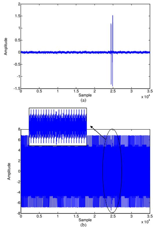
Fig. 3. (a) The output of the sensor due to two consecutive metallic particle passages (Particles: ferromagnetic, diameter = 175  $\mu\text{m}$  and non-ferromagnetic, diameter = 508  $\mu\text{m}$ ) (b) Output Signal +  $2 \sin(1400\pi t)(1 + \cos(900\pi t)) + 2 \sin(2000\pi t)(1 + \cos(700\pi t))$
