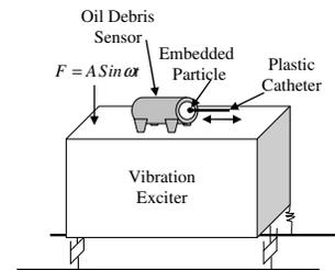
Fig.9 Schematic of test setup.
