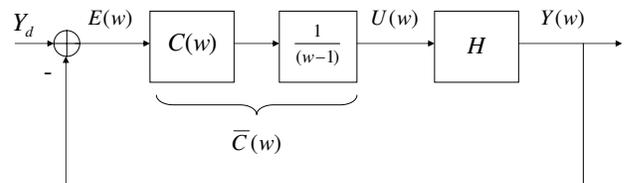
Fig. 1. Standard ILC setup in the supervector framework.
