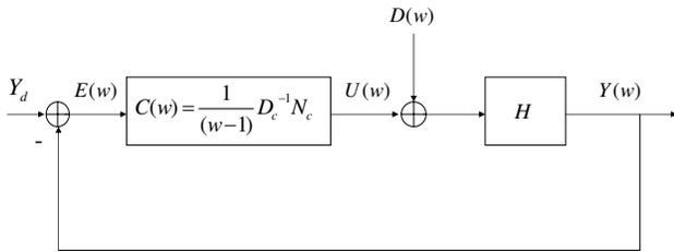
Fig. 4.  $l_1$  problem framework using an integrating controller.
