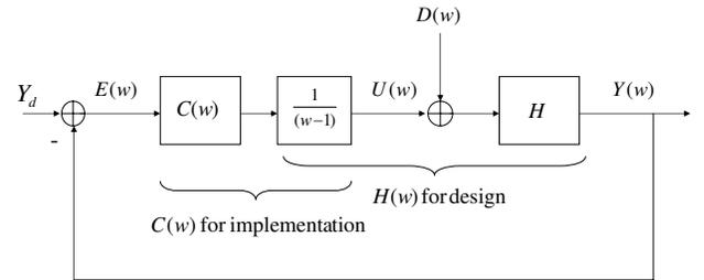
Fig. 5.  $l_1$  problem framework using an integrating plant.
