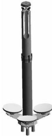
Figure 2: Deployable Optical Telescope
