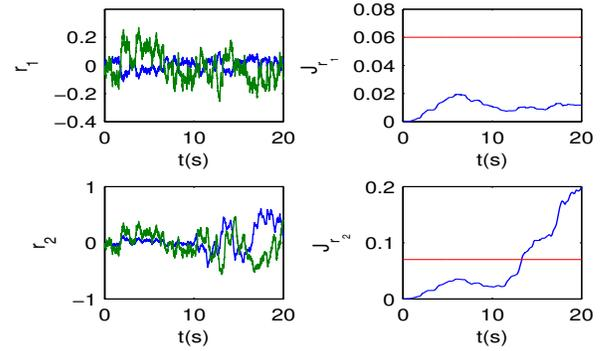
Fig. 2. Residual signals and their evaluation functions corresponding to a fault in the second actuator.
