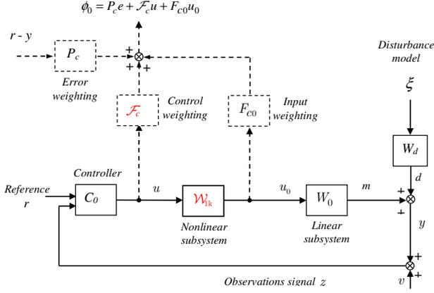
Fig.1 Two Degrees of Freedom Feedback Control for Nonlinear Plant
