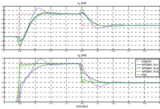
Fig. 6: Position control for varying  $N$ : angles
