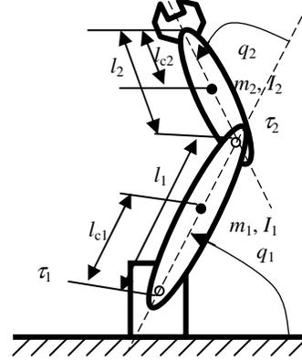
Fig. 5: Two-link robotic manipulator
