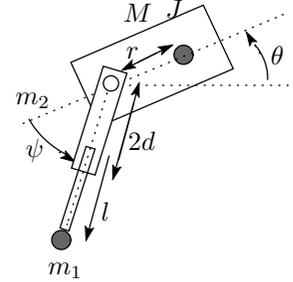
Fig.1. Flying robot with extending and contracting lower limbs
