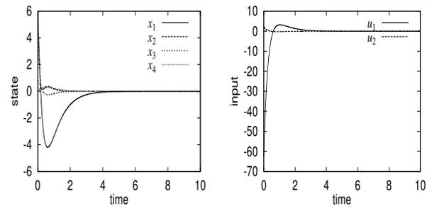
$$\begin{aligned} \text{(a)} \quad \mathbf{x}(0) &= [6, 5, \pi/4, 0]^T \\ \mathbf{u}_0 &= [-62.31, 2.023]^T \end{aligned}$$
