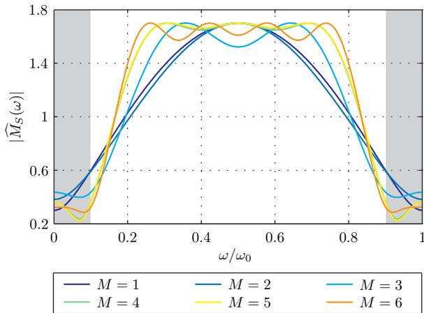
Fig. 6. Optimal  $\widehat{M}_S(\omega)$  for  $L\Delta = 10\%$ ;  $\gamma_{np} = 1.7$  and different orders  $M$  of the repetitive controller. The grey band indicates the uncertainty interval  $\widehat{\Omega}_L$ .
