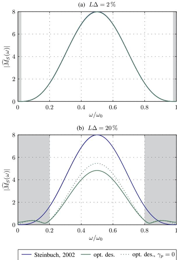
Fig. 8. Comparison of optimal repetitive control design and the repetitive controller designed by Steinbuch (2002) for  $M = 3$ : (a)  $L\Delta = 2\%$ ; (b)  $L\Delta = 20\%$ . In figure (b) the optimal solution with  $\gamma_p = 0$  as additional constraint is also shown. The grey band indicates the uncertainty interval  $\Omega_L$ .
