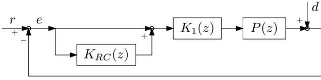
Fig. 2. Control setup of an add-on repetitive control system.
