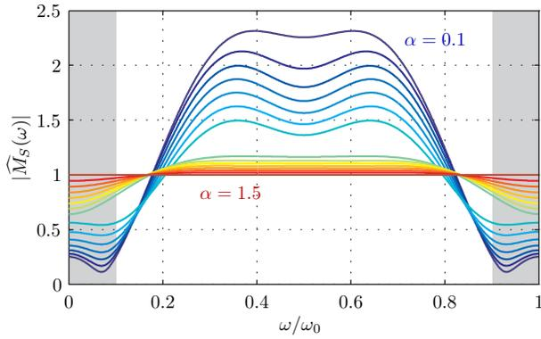
Fig. 5. Optimal  $\widehat{M}_S(\omega)$  for  $M = 3$  and  $L\Delta = 10\%$ ;  $\alpha$  ranges from 0.1 to 1.5 with an increment of 0.1. The grey band indicates the uncertainty interval  $\widehat{\Omega}_L$ .
