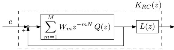
Fig. 3. Structure of a high-order repetitive controller.
