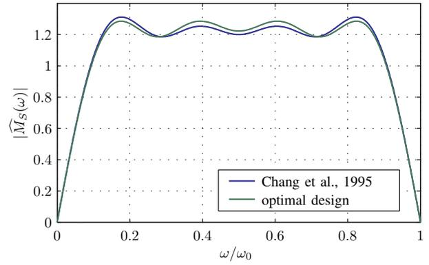
Fig. 7. Comparison of optimal repetitive control design ( $\alpha = 10^{-3}$ ) and the repetitive controller designed by Chang et al. (1995) for  $M = 4$ .
