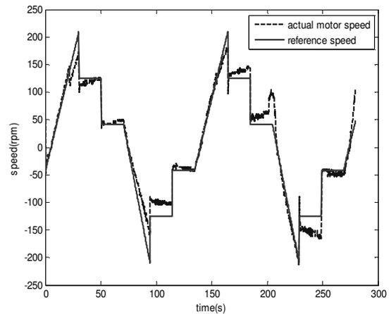
Fig.(13) Performance of the one step ahead controller for Experiment 3
