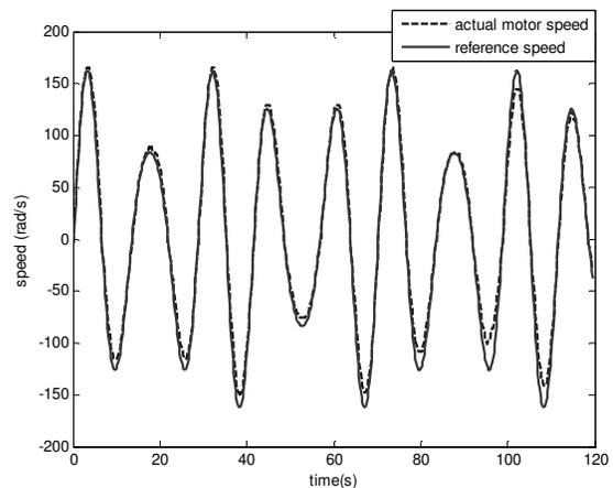
Fig.(9) Performance of the linear controller for Experiment 2
