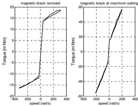
Fig.(7) Torque-speed characteristics of the load.
