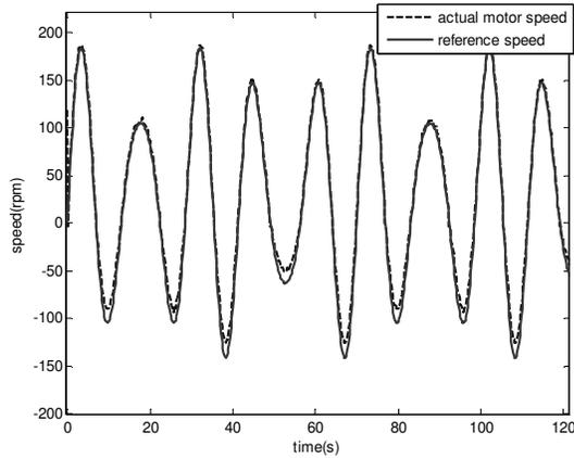
Fig.(10) Performance of the one step ahead controller for Experiment 2
