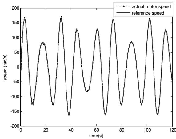
Fig.(11) Performance of the inverse controller for Experiment 2
