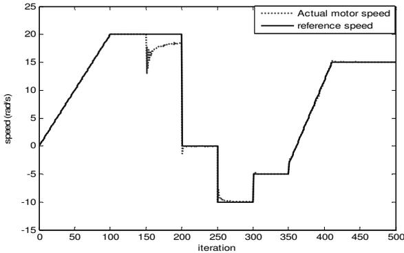
Fig.(3) response of the one step ahead controller Experiment 1.
